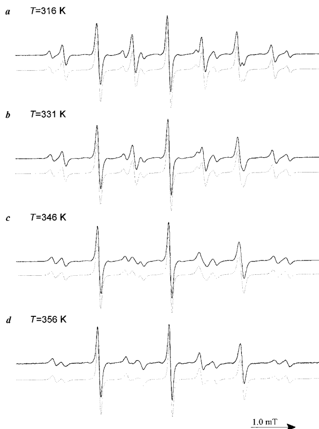
Figure 2. EPR spectra of nitroxide 1a recorded in water in the presence of 3.25 \times 10^{-3} \text{ M} \beta -CD at different temperatures. The dotted lines show the corresponding simulations. a) k_1 = 1.0 \times 10^9 \text{ M}^{-1} \text{ s}^{-1} , k_{-1} = 1.6 \times 10^6 \text{ s}^{-1} ; b) k_1 = 1.5 \times 10^9 \text{ M}^{-1} \text{ s}^{-1} , k_{-1} = 2.9 \times 10^6 \text{ s}^{-1} ; c) k_1 = 2.0 \times 10^9 \text{ M}^{-1} \text{ s}^{-1} , k_{-1} = 5.1 \times 10^6 \text{ s}^{-1} ; d) k_1 = 2.3 \times 10^9 \text{ M}^{-1} \text{ s}^{-1} , k_{-1} = 8.7 \times 10^6 \text{ s}^{-1} . As an example, spectrum (b) was simulated by assuming the presence of the free species (37%) in the bulk aqueous phase ( g factor 2.0056, linewidth 0.029 mT, a(9\text{H}) 0.018 mT, a(\text{N}) 1.659 mT, a(2\text{H}) 1.031 mT), and the included radical (63%) ( g factor 2.0058, linewidth 0.031 mT, a(9\text{H}) 0.018 mT, a(\text{N}) 1.584 mT, a(2\text{H}) 0.802 mT).
